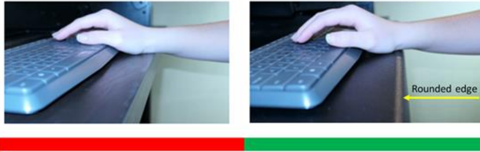
Figure: 6: Rounded edges (right panel) are better; photo from NIOSH
